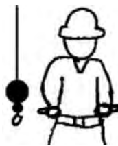
EXTEND TELESCOPING BOOM – With hands to the front at waist level, thumbs point outward with other fingers closed.
