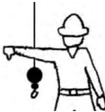
LOWER BOOM – With arm extended horizontally to the side, thumb points down with other fingers closed.
