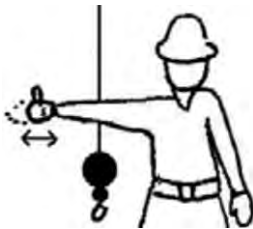
RAISE THE BOOM AND LOWER THE LOAD – With arm extended horizontally to the side and thumb pointing up, fingers open and close while load movement is desired.
