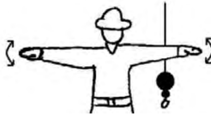
EMERGENCY STOP – With both arms extended horizontally to the side, palms down, arms are swung back and forth.
