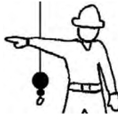
SWING – With arm extended horizontally, index finger points in direction that boom is to swing.
